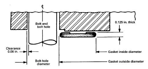
TABLE 21 JACKETED GASKET DIMENSIONS FOR ASME B16.5 FLANGES
